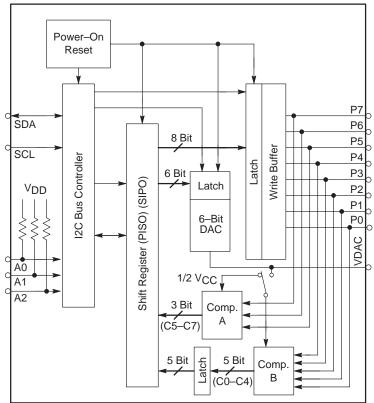
NOTE: Internal Power On Reset sets P0  $\sim$  P7 low, sets VDAC to 1/80 VDD and selects 1/2 V<sub>DD</sub> for Comparator "B" threshold.
